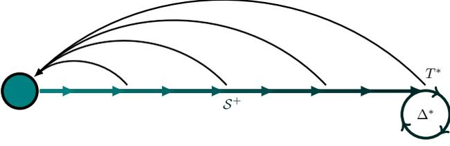
FIG. 5.  $\epsilon$ -Machine for an eventually  $\Delta$ -Poisson renewal process: Graphical elements as in the previous figure. The circular causal-state space at  $T^*$  (circle on right) has total duration  $\Delta^*$ , corresponding to any time since last event after  $T^*$  mod  $\Delta^*$ . If no event is seen, probability flows as indicated around the circle, as described in Eq. (6).
