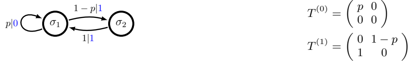
FIG. 1: A hidden Markov model (the \epsilon -machine) for the Even Process. The support for this process consists of all binary sequences in which blocks of uninterrupted 1s are even in length, bounded by 0s. After each even length is reached, there is a probability p of breaking the block of 1s by inserting a 0. The machine has two internal states \mathcal{S} = \{\sigma_1, \sigma_2\} , a two symbol alphabet \mathcal{X} = \{0, 1\} , and a single parameter p \in (0, 1) that controls the transition probabilities. The associated Markov chain over states is finite-state and irreducible and, thus, has a unique stationary distribution \pi = (\pi_1, \pi_2) = (1/(2-p), (1-p)/(2-p)) . The graphical representation of the machine is given on the left, with the corresponding transition matrices on the right. In the graphical representation the symbols labeling the transitions have been colored blue , for visual contrast, while the transition probabilities are black.
