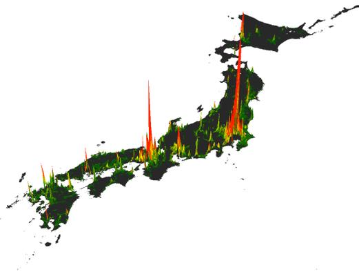
**Figure 1.** Spatial distribution of material stocked in buildings for 2009. Generated from data from Fishman et al.<sup>3,4</sup>
