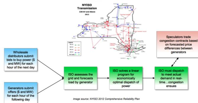
**Figure 1.** ISO Process and New York transmission grid
