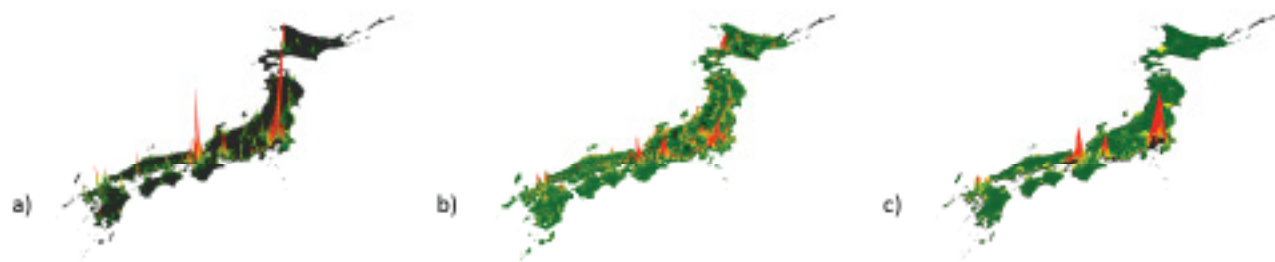
Figure 1. Spatial distribution of a) material stocked in buildings for 2009, b) material stocked in roads in 2010, and c) population. Generated from data from Fishman et al. (2014) and Turchiova et al. (2015).
